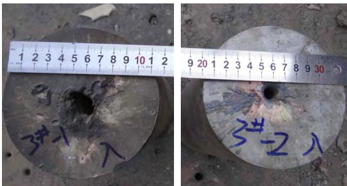
Figure 14: The experimental results PTFE jet and PTFE/Cu jet penetrating main armour.
