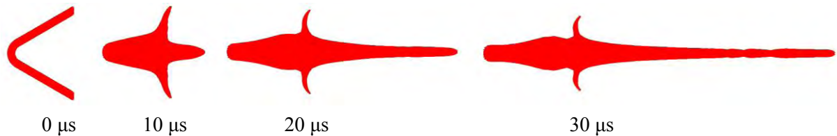
Figure 2: Numerical simulation of the formation of PTFE/Cu at different time.
