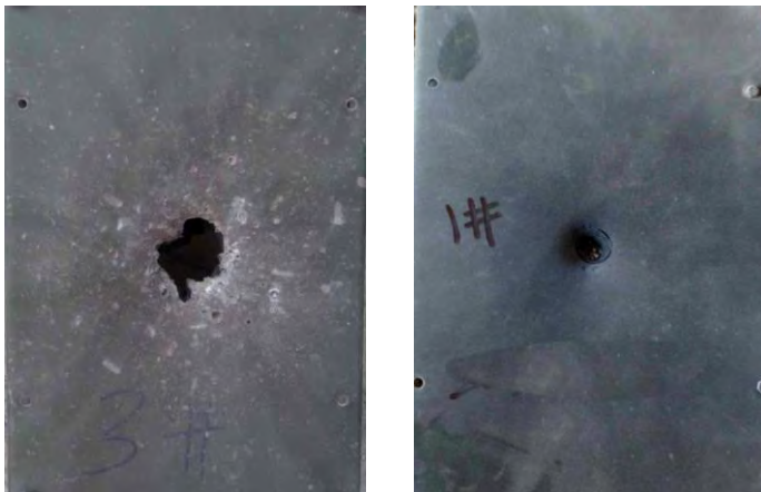
Figure 13: The experimental results PTFE jet and PTFE/Cu jet penetrating shell charge.
