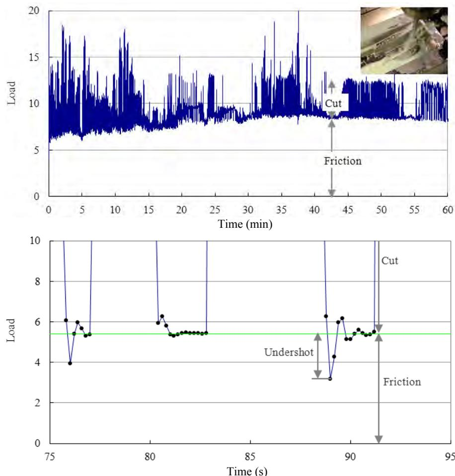
Figure 6: Slow friction load change (top) and undershot noise (bottom).
