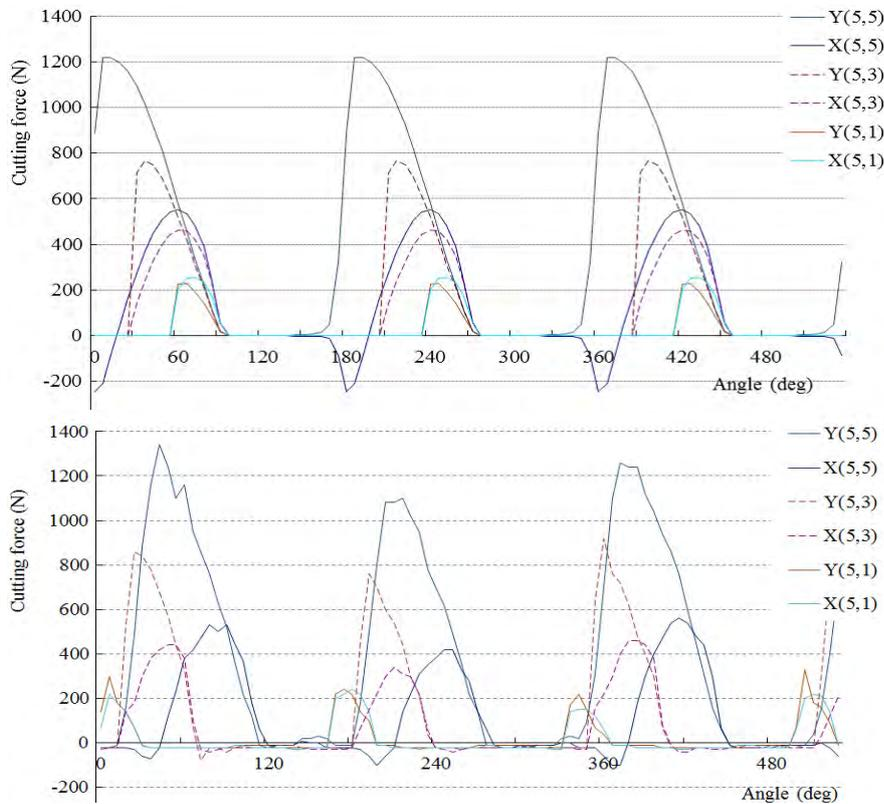
Figure 2: Predicted (top) and measured (bottom) instantaneous cutting forces.
