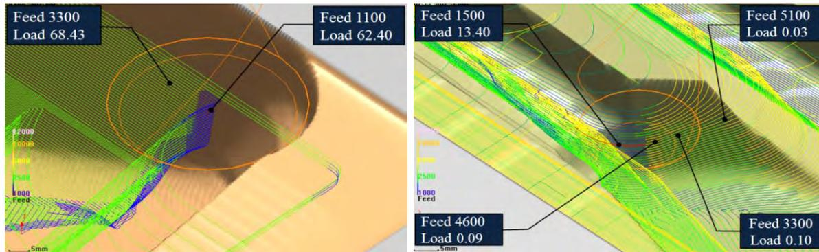
Figure 8: Pre-simulation at the roughing (left) and re-roughing (right) step.
