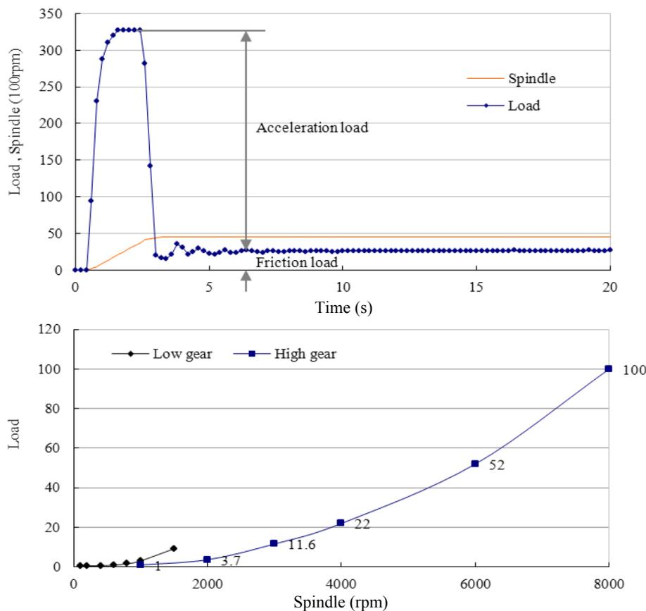
Figure 5: Spindle acceleration load (top) and friction load (bottom).
