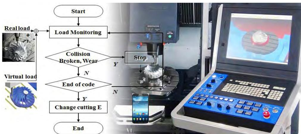
Figure 13: Pre-simulation and sensorless monitoring integrated in an open CNC.
