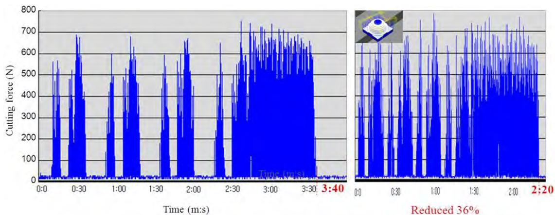
Figure 3: Pre-control feed rate to save machining time.
