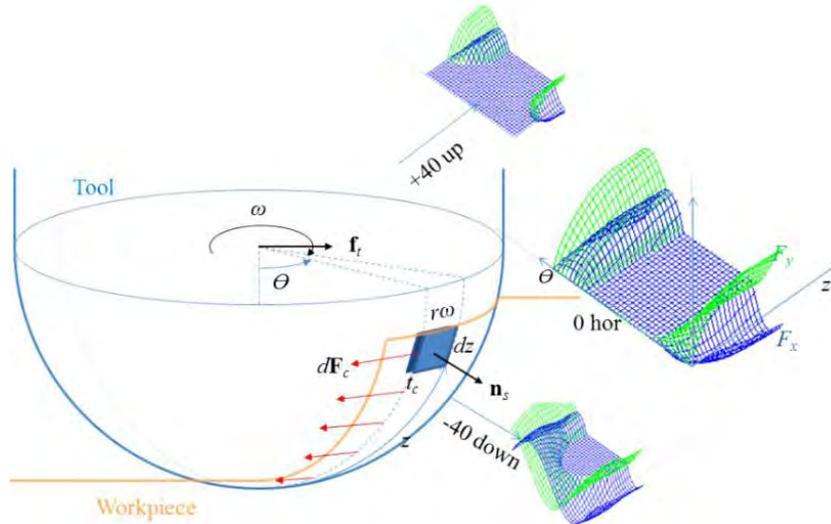
Figure 1: Element cutting forces on a tool.
