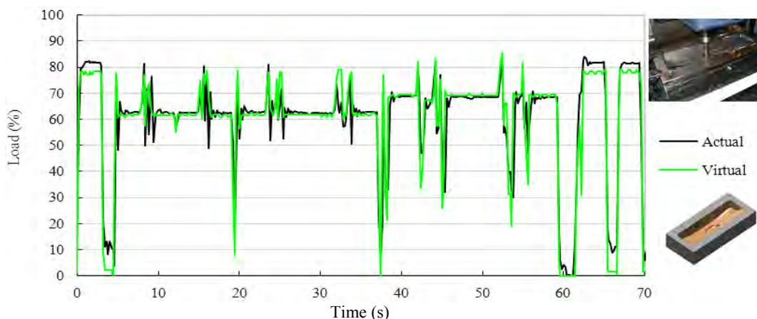
Figure 9: Roughing by a  $\Phi 50$ -mm cutter.
