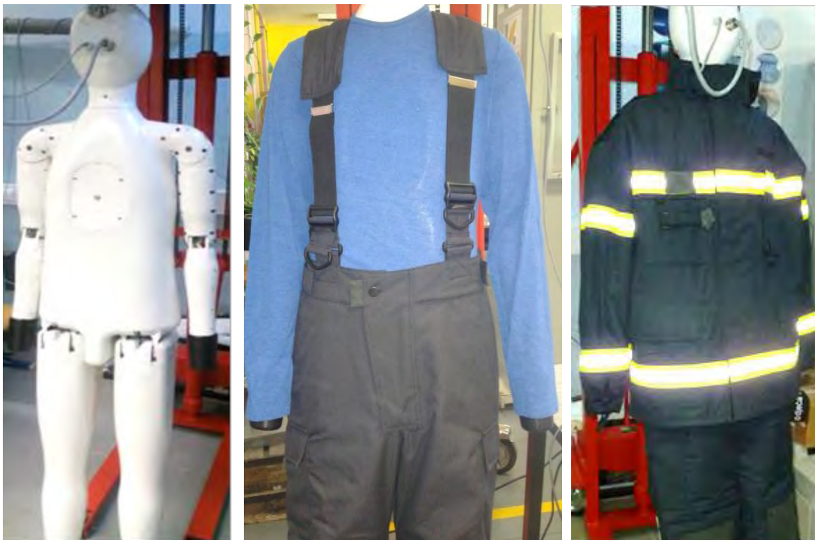
Figure 4: Thermal manikin – naked and dressed (with underwear and in a firefighter suit).
