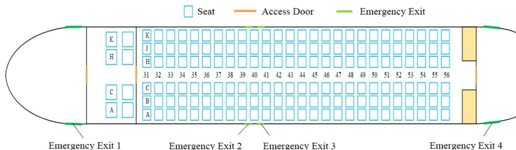
Figure 1: Cabin structure of B737-800 configuration A.
