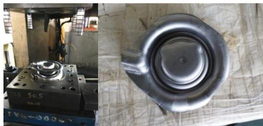
Figure 11: Forming die and work piece.
