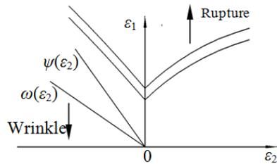
Figure 4: Diagram of forming limit.
