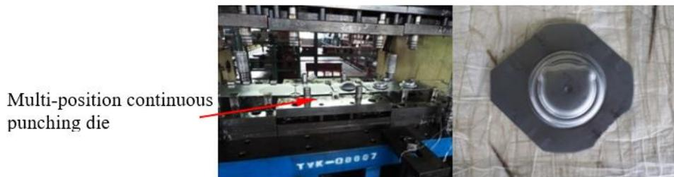
Figure 10: Continuous-punching die and work piece.
