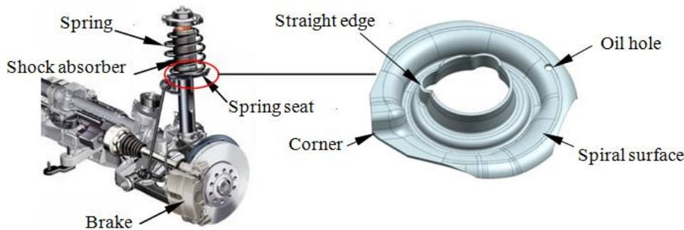
Figure 1: Diagram of suspension system and model of spring seat.
