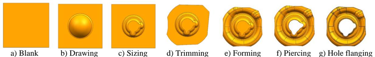
Figure 2: Multi-step stamping process of spring seat.
