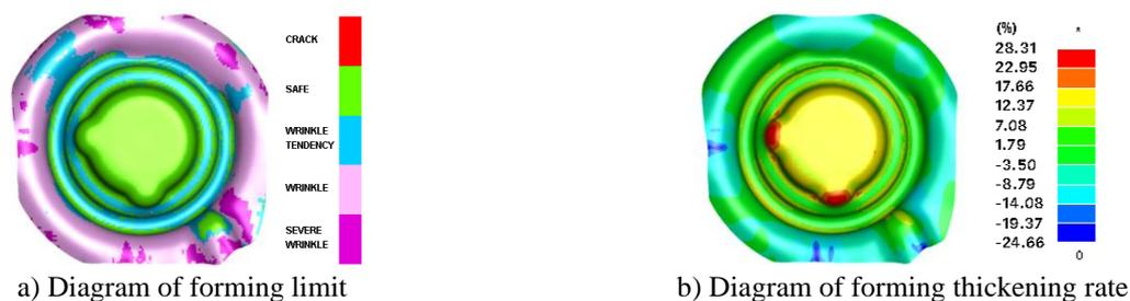
Figure 5: Defect analysis of forming process before optimisation.
