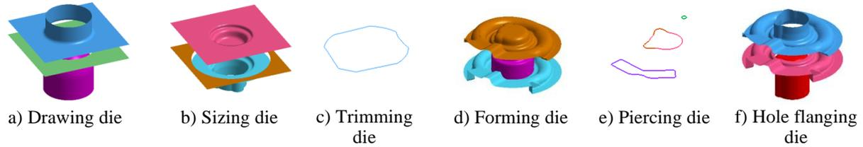
Figure 3: Dies for multi-step stamping process.
