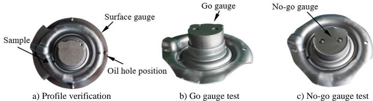
Figure 13: Gauges for detecting.
