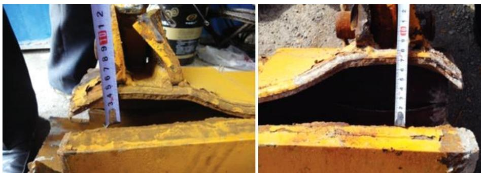
Figure 1: Problems of welding seams on a tower crane.
