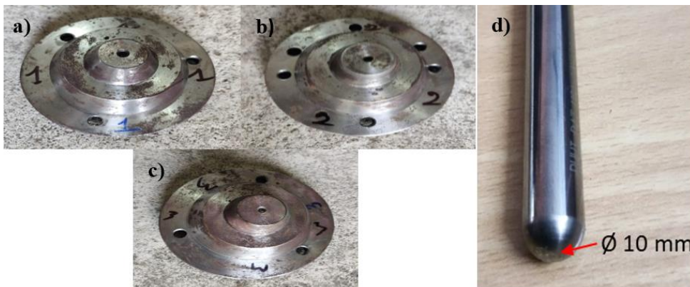
Figure 2: a), b) and c) TPIF forming dies with 70^\circ , 73^\circ and 75^\circ top wall angles, d) forming tool.
