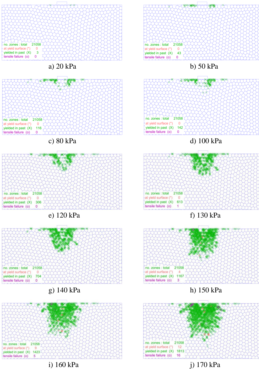
Figure 6: The distribution of the plastic zone of soil mass under different load.
