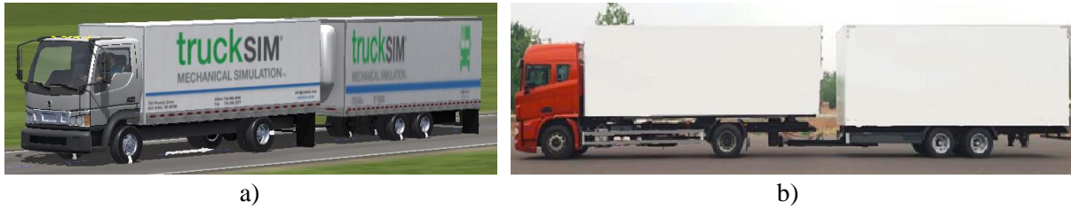
Figure 2: a) 3-D TruckSim model, b) testing truck-CAT combination.
