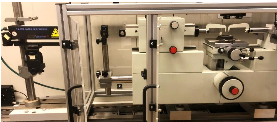
Figure 1: Calibration of the ring diameter on a universal 1D machine by applying laser interferometer as a standard.
