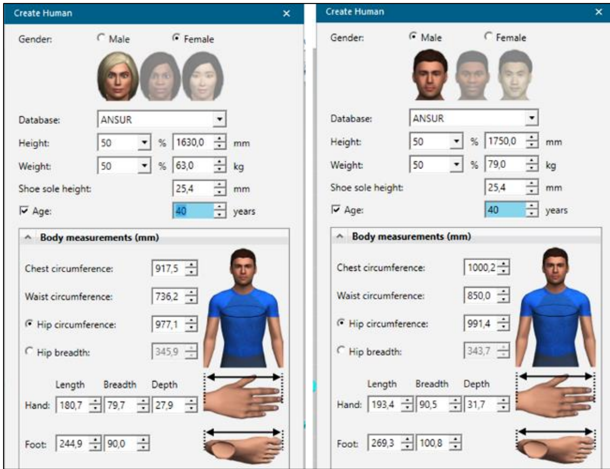
Figure 3: Human Avatar characteristics used in Process Simulate.
