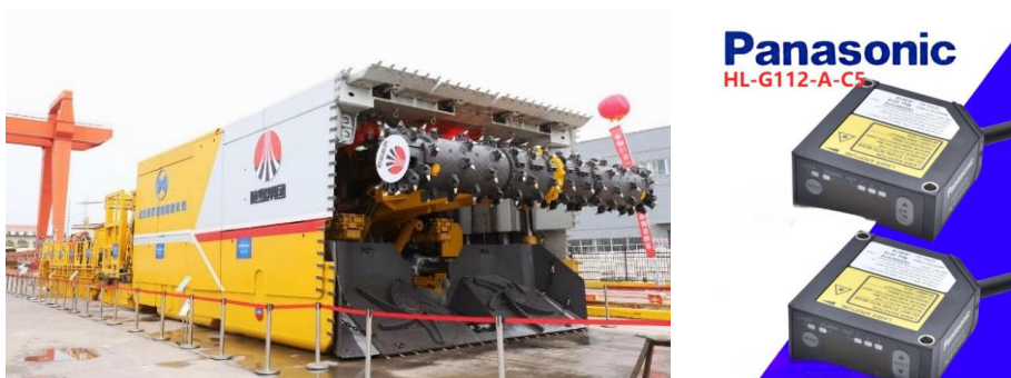
Figure 10: Rapid tunnelling system and laser displacement sensors.
