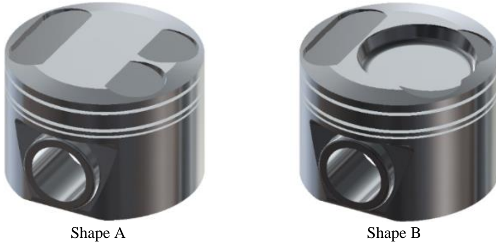
Figure 3: Piston shape comparison (shape A – flat-shaped piston; shape B – bowl-shaped piston).
