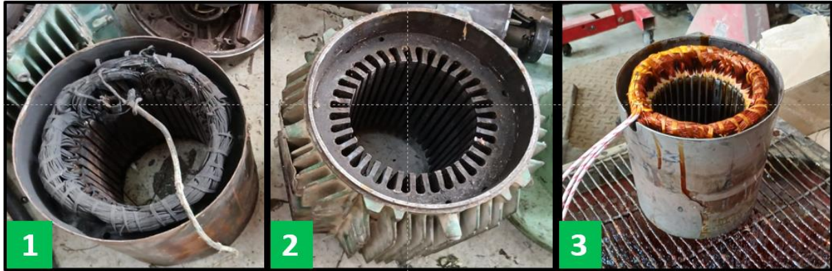
Figure 3: Motor core before the unwinding step (1), after unwinding step (2), and after the rewinding step (3).
