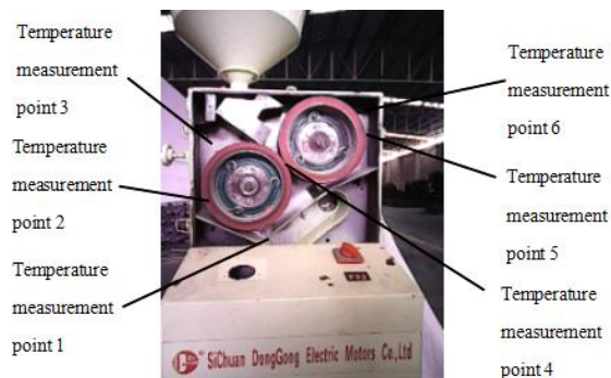
Figure 1: Schematic diagram of temperature detection point in the hulling chamber.
