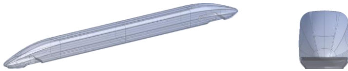
Figure 2: Geometric model of the train: train side view (left), train front view (right).
