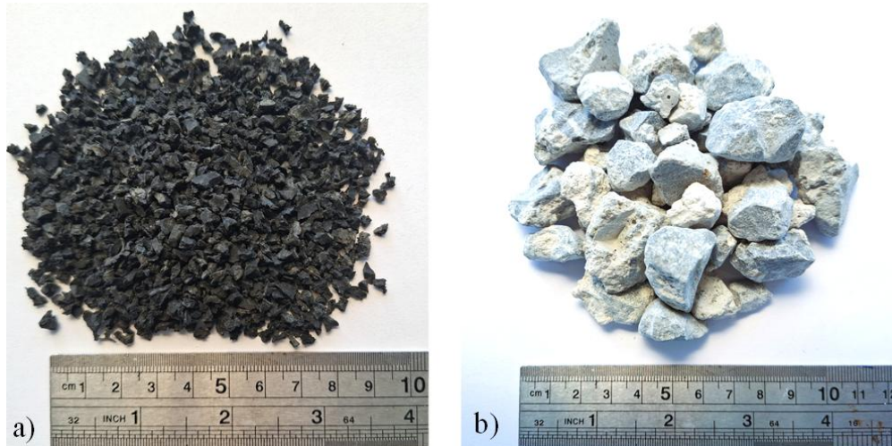
Figure 1: a) crumb rubber, b) recycled concrete aggregate.
