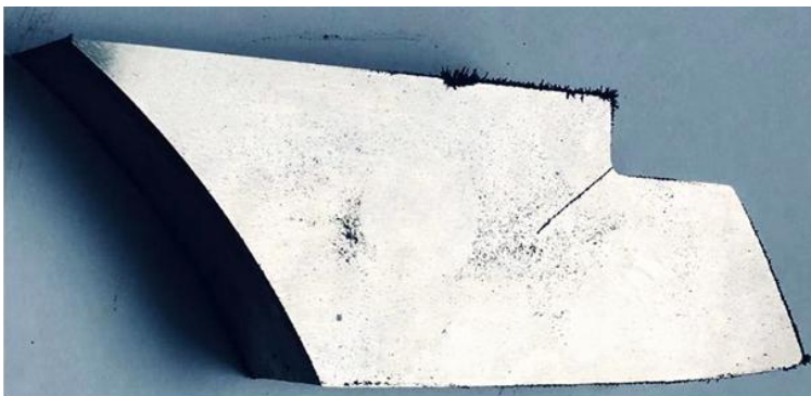
Figure 11: Cracks that occur at the transition R position on the other side.
