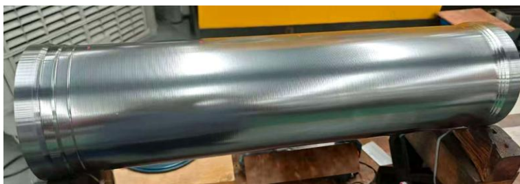
Figure 9: The workpiece after the spinning process is completed.
